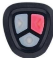
**Right turn light button:** Press once, then the light will flow to the right, and press the light again to turn off the light in a short time and then return to the original mode.
