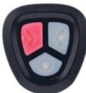
**Left turn light button:** Press once, then the light will flow to the left, and press the light again to turn off the light in a short time and then return to the original mode.
