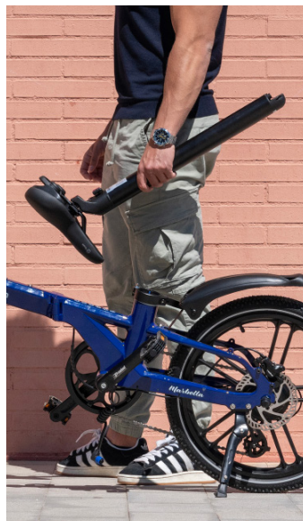
battery integrated into the seat post
