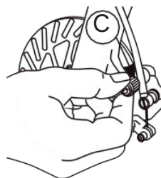
Fig. 15 Disc brake pads adjustment
